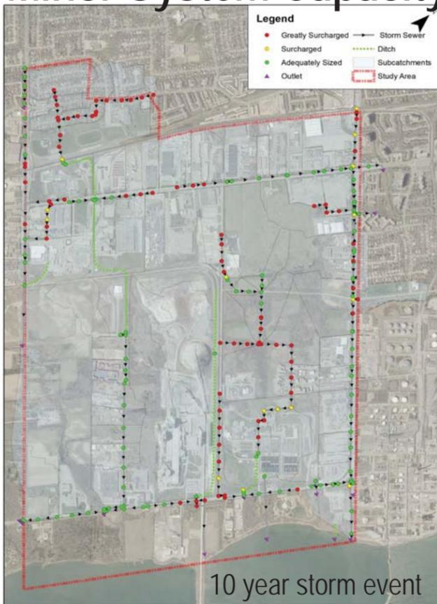
Storm sewer segments illustrated in green are big enough to meet the City's capacity standards under the current landuses. Sewer segments illustrated in red are undersized which may cause stormwater to "backup" and pond on the road.
